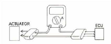
The assortment of Round and Flat Terminal or Socket connector cables can be used as a breakout connection for measuring signals with test equipment.
