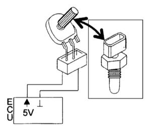
Simulating the temperature sensor signal;
