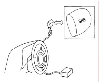
**Note:** The SRS (Airbag) Plug is fused at 0.25 Amps. If the current supply is over this rating, its fuse will blow.
