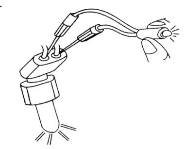
Detecting the injection pulse signal
