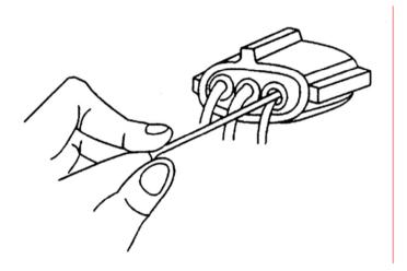
Needle probe used at the sensor connector end
